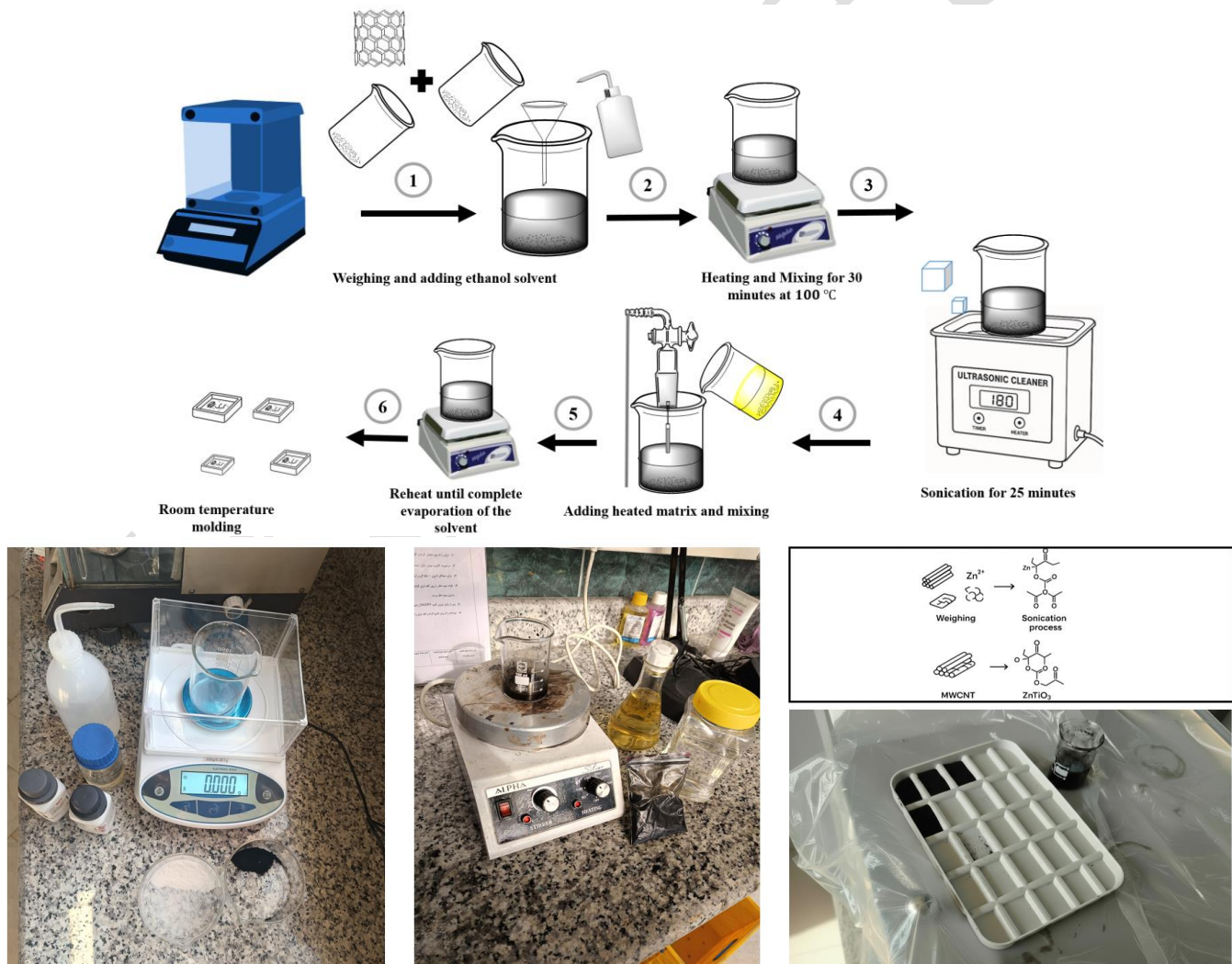
Fig. 4. Experimental procedure for laboratory-scale nanocomposite fabrication
